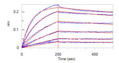
Loaded SARS-CoV-2 S1 protein, Mouse IgG2a Fc Tag (Cat. No. S1N-C5257) on AMC Biosensor, can bind Human ACE2, His Tag (Cat. No. AC2-H52H8) with an affinity constant of 2.53 nM as determined in BLI assay (ForteBio Octet Red96e) (Routinely tested).
