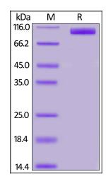
Human ACE2, His Tag on SDS-PAGE under reducing (R) condition. The gel was stained with Coomassie Blue. The purity of the protein is greater than 95%.
