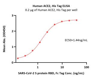
Immobilized Human ACE2, His Tag (Cat. No. AC2-H52H8) at 2  $\mu$ g/mL (100  $\mu$ L/well) can bind SARS-CoV-2 S protein RBD, Fc Tag (Cat. No. SPD-C5255) with a linear range of 0.2-5 ng/mL (Routinely tested).
