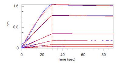
Loaded Biotinylated Mouse BCMA, Fc, Avitag (Cat. No. BCA-M82F0) on SA Biosensor, can bind Human APRIL, His, Flag Tag, active trimer (Cat. No. APL-H52D1) with an affinity constant of 2.19 nM as determined in BLI assay (ForteBio Octet Red96e) (Routinely tested).
