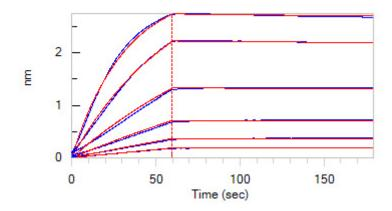
Loaded Biotinylated Mouse BCMA, Fc, Avitag (Cat. No. BCA-M82F0) on SA Biosensor, can bind Mouse BAFF, Mouse IgG2a Fc Tag, low endotoxin (Cat. No. BAF-M5257) with an affinity constant of 3.75 nM as determined in BLI assay (ForteBio Octet Red96e) (Routinely tested).
