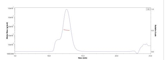
The purity of Mouse CEACAM-5, Fc Tag (Cat. No. CE5-M5253) is more than 85% and the molecular weight of this protein is around 280-360 kDa verified by SEC-MALS.
