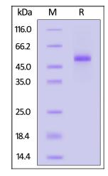
Biotinylated Cynomolgus DLL3, His, Avitag on SDS-PAGE under reducing (R) condition. The gel was stained with Coomassie Blue. The purity of the protein is greater than 95%.
