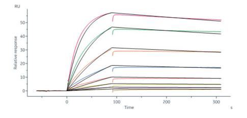
Anti-Factor XI Antibody captured on Protein A Chip can bind Human Coagulation factor XI, His Tag (Cat. No. FXI-H52H5) with an affinity constant of 15.2 nM as determined in a SPR assay (Biacore 8K) (Routinely tested).
