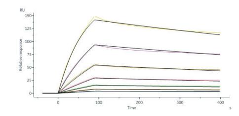
GMP Biotinylated Human DLL4 Protein, His,Avitag (Cat. No. GMP-DL4H23) immobilized on CM5 Chip can bind Human NOTCH1 Protein, Fc Tag (Cat. No. NO1-H5255) with an affinity constant between 1.00 nM - 30.0 nM as determined in a SPR assay (Biacore 8K) (QC tested).
