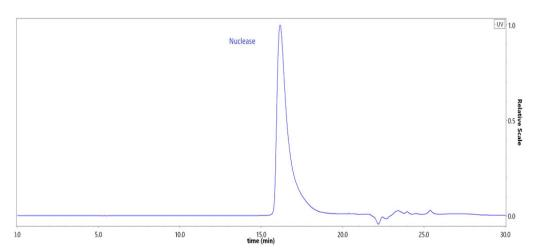
The purity of GMP GENIUS<sup>TM</sup>Nuclease (Cat. No. GMP-NUES19) was greater than 99% as determined by SEC-HPLC.
