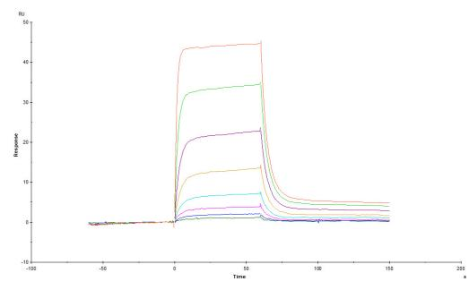
Human IL-2 R beta, Fc Tag (Cat. No. ILB-H5253) captured on CM5 chip via anti-human IgG Fc antibody can bind IL-2, Tag Free with an affinity constant of 0.473  $\mu$ M as determined in a SPR assay (Biacore T200) (QC tested).
