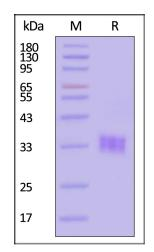
Human PD-L1, His Tag on SDS-PAGE under reducing (R) condition. The gel was stained with Coomassie Blue. The purity of the protein is greater than 98% (With Star Ribbon Pre-stained Protein Marker).
