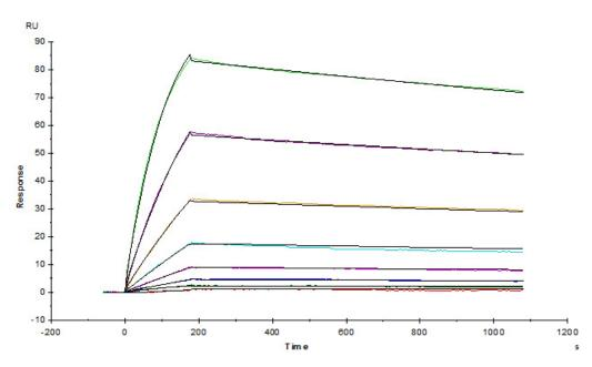
Anti-Human PD-L1 Mab (Human IgG1) captured on CM5 chip via anti-human IgG Fc antibodies surface, can bind Human PD-L1, His Tag (Cat. No. PD1-H5229) with an affinity constant of 0.286 nM as determined in a SPR assay (Biacore T200) (Routinely tested).
