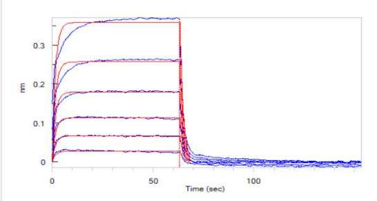
Loaded Human PD-1, Fc Tag, low endotoxin (Cat. No. PD1-H5257) on ProteinA Biosensor, can bind Human PD-L1, His Tag (Cat. No. PD1-H5229) with an affinity constant of  $5.3~\mu M$  as determined in BLI assay (ForteBio Octet Red96e) (QC tested).
