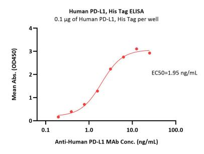
Immobilized Human PD-L1, His Tag (Cat. No. PD1-H5229) at 1  $\mu$ g/mL (100  $\mu$ L/well) can bind Anti-Human PD-L1 MAb (Human IgG1) with a linear range of 0.1-3 ng/mL (QC tested).
