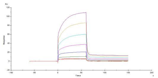
Human PD-1, Fc Tag (Cat. No. PD1-H5257) captured on CM5 chip via antihuman IgG Fc antibody, can bind Human PD-L1, His Tag (Cat. No. PD1-H5229) with an affinity constant of 3.6  $\mu$ M as determined in a SPR assay (Biacore T200) (Routinely tested).
