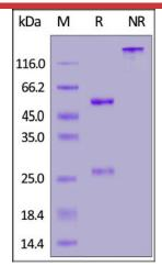
Anti-SARS-CoV-2 Spike RBD Antibody, Chimeric mAb, Human IgG1 (AM122) on SDS-PAGE under reducing (R) and non-reducing (NR) conditions. The gel was stained with Coomassie Blue. The purity of the protein is greater than 95%.
