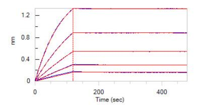
Loaded Biotinylated Mouse VEGF164, His, Avitag (Cat. No. VE4-M82Q3) on SA Biosensor, can bind Mouse VEGF R1 Protein, Mouse IgG2a Fc Tag (Cat. No. VE1-M5256) with an affinity constant of 42.4 pM as determined in BLI assay (ForteBio Octet Red96e) (Routinely tested).
